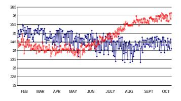
The data was imported into the web based application, which then carried out various probability matches - see below. The DataReader correctly diagnosed root induced clay shrinkage as the most likely cause of movement.
